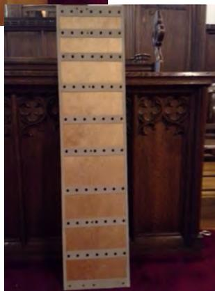
This picture shows a bottom board after it was flattened. The small holes on the top of the board connect to the individual pneumatics. The larger holes on the end of the board connect to the note channel, which extends the length of the board. Each board was made in two pieces. The note channels were routed out on each of piece, and then the two pieces glued together.
