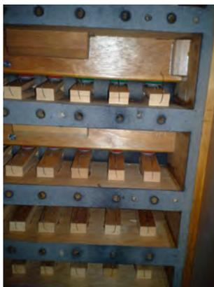
This picture shows the inside of the chest with the pipe pneumatics. Each pneumatic controls one note of one stop. Considering that there are 61 notes on the keyboards, and 20 stops (11 on the Swell, 9 on the Great), that makes a grand total of 1220 pneumatics!
